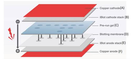
**Important note about the sandwich:** The current will flow from the negatively charged cathode (black) to the positively charged anode (red). The proteins within your gel are negatively charged because you added SDS to help denature
