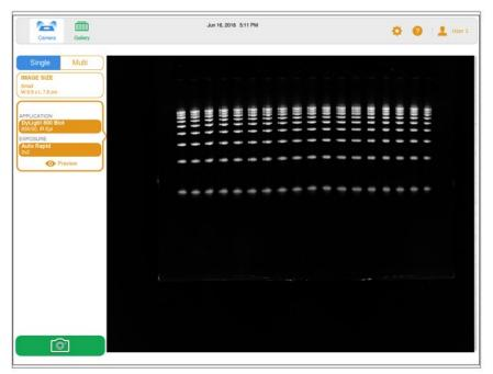
8.4.7 Once any necessary adjustments have been made, click the camera icon in order to acquire an image of your membrane
