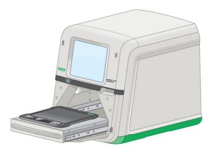
8.4.3. Place your membrane on the **Blot/UV/Stain-free tray.** If the try is not in the rack it may be in the instrument. Gently open the imaging system and pull out the tray; place your membranes so that the side with visible bands is facing upwards at you
