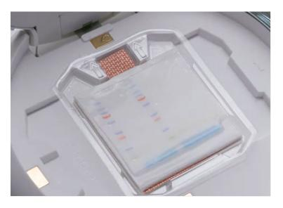
8.1.5. Briefly soak a piece of filter paper in DI water, then place the filter paper on top of your gel. Use the roller to remove air bubbles.
