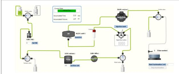
Figure 3. Example flow path (REF: AKTA Start User manual)<sup>9</sup>. Sample is loaded into injection valve and kept in the sample loop. Once ready Buffer pumped from A, B, or a mixture of either can be passed across the sample loop, pushing the sample through the remainder of the system.
