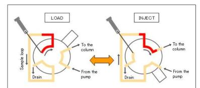
Figure 4. The two changing flow paths of the sample loop. When the system is set to "LOAD," sample can be loaded into the sample loop. When the system is set to "INJECT," it is ready for buffer to pass through the loop and inject the sample into the downstream components of the system (Source: Hitachi. Configuration of HPLC System.)<sup>11</sup>
