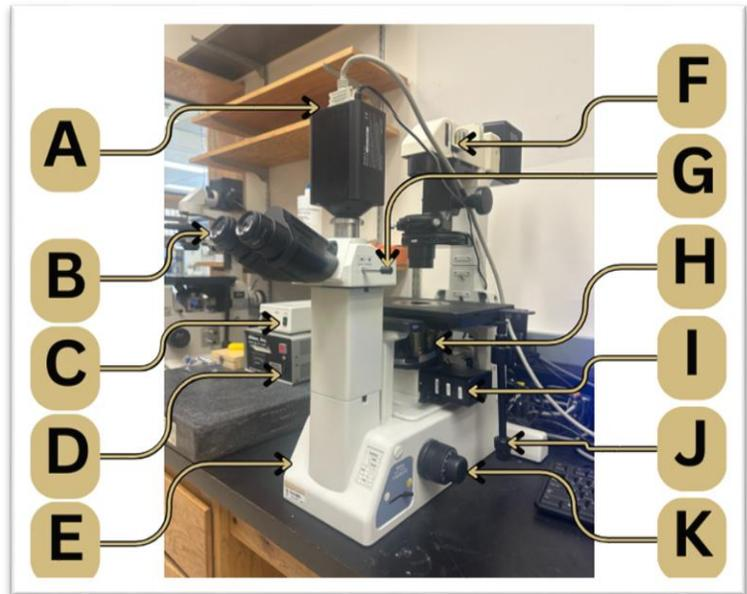
*Figure 2. Nikon Eclipse TE-200 Microscope. (A) labels the camera. (B) labels the eyepiece. (C) labels the on/off for brightfield lamp. (D) labels the on/off for UV fluorescence lamp. (E) labels the on/off for brightfield. (F) labels the on/off for brightfield illumination. (G) labels the switch for eyepiece/camera viewing. (H) labels the objective lens carousel. (I) labels the fluorescence filter selector. (J) labels the stage controls. (K) labels the focus knob.*
