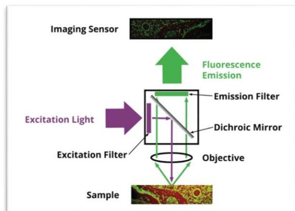
Figure 1. An illustration of how the filter cube functions to excite a sample and detect the emitted fluorescence. (DOVERMOTION, n.d)
