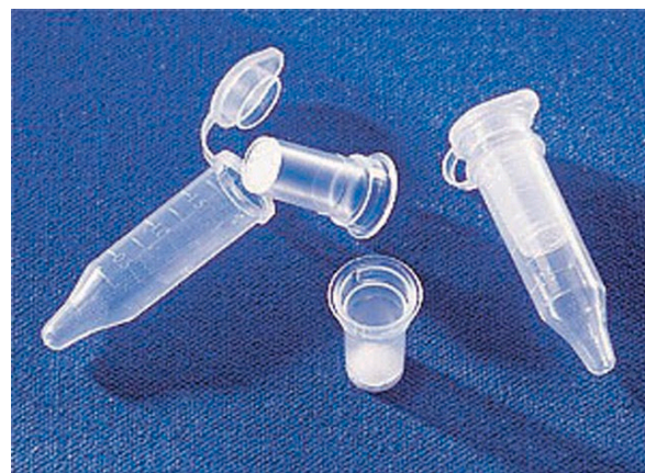
Figure 1. Microcentrifuge spin filters. The filter (small well with silica membrane) is placed inside a microcentrifuge tube. Centrifugation passes solutions through the filter and the eluant collects at the bottom of the microcentrifuge tube.
