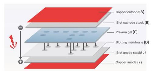
**Important note about the sandwich:** The current will flow from the negatively charged cathode (black) to the positively charged anode (red). The proteins within your gel are negatively charged because you added SDS to help denature them. Therefore, the proteins will move towards the anode, making it imperative that you correctly assemble the sandwich.
