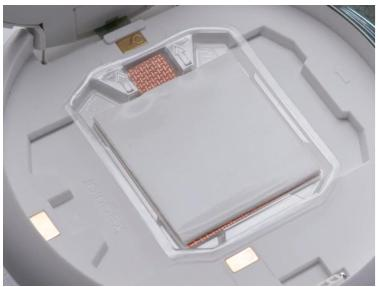
8.1.4. Carefully pick up your pre-run SDS-PAGE gel and place it on the membrane
