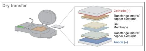
Figure 4. Dry transfer. Dry transfers do not use transfer buffer at all; rather, the gel is placed between preassembled transfer stacks containing the transfer membrane and necessary components to successfully transfer your blot from your gel to the membrane.
